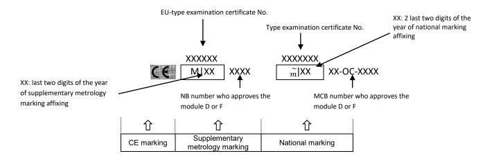
The CE marking, the supplementary metrology marking and national marking, as appropriate, shall be affixed visibly, legibly and indelibly to the measuring instrument or to its data plate. Where that is not possible or not warranted on account of the nature of the measuring instrument, they shall be affixed to the accompanying documents and to the packaging, if any.
